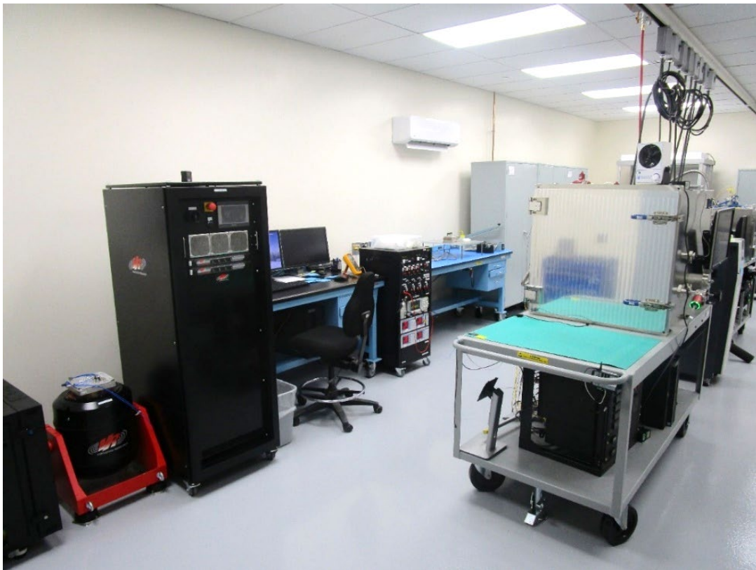
Figure 1. New space CCE integration and test area at Creare. The area is equipped with two thermal vacuum chambers, a shaker table, bakeout chambers, and clean assembly and test benches.
